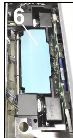
7. **Close Printhead Latch [6].** Printer starts up and primes ink into Printhead. (*This may take a few minutes.*) Make sure ink is flowing through hoses. If air bubbles appear, tap lines or click **“Circulate Ink”** on Touchscreen to clear them.
