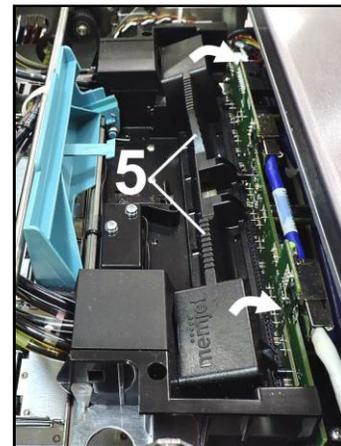
5. **Close Printhead Latch [6].** Printer starts up and primes ink into Printhead (*this may take a few minutes.*) Make sure ink is flowing through hoses.
